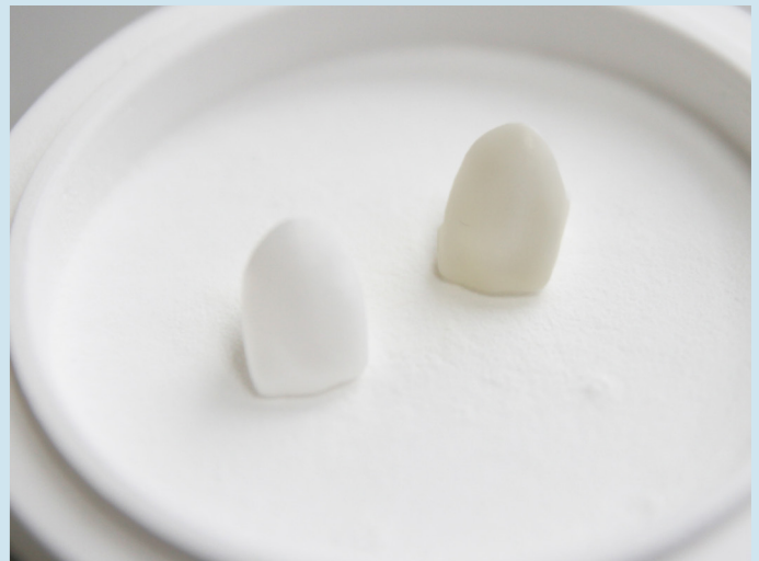
Fig. 1: Exemplary contamination of white material. The left crown is sintered in a pure furnace atmosphere, the right crown in a contaminated environment. The effect of coloring metal ions is clearly visible.
